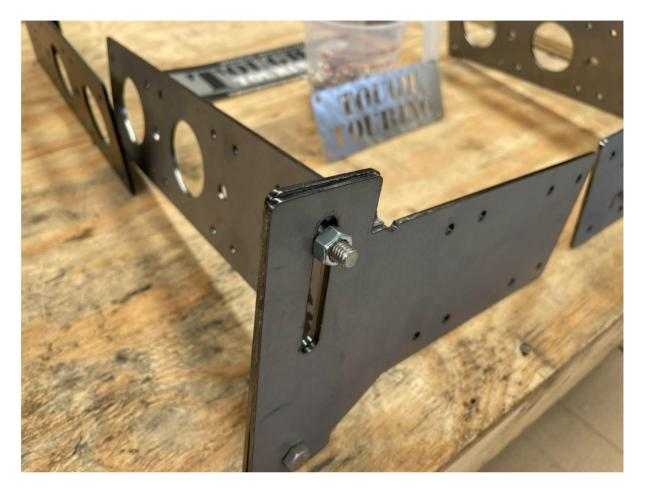
9. Repeat process of lining up the front bracket above – same as you did for the rear, positioning the bracket about 3mm down from the aluminium edge plate on the tent – Position your - again tec screw it into position as a 'test fit' using 2 tec screws. Check that it sits level. And square. AGAIN - Make sure the triangular section of the bracket is facing downwards... The Lid of the tent need to be able to shut without hitting the brackets ...
