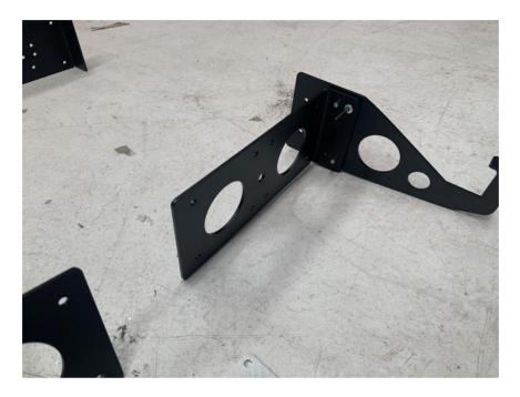
11. There is a blank plate included in the kit for the front driver's side. Its useful to balance up the look of the bracket kit and complete the install, it also proves handy if your going to add any lifting eyebolts etc that come in out Cradle mount (Removable tent) options kit. The blank steel plate there also can be helpful at protecting that edge of the tent from tree strikes etc. See blank plate for Front drivers' side below.
