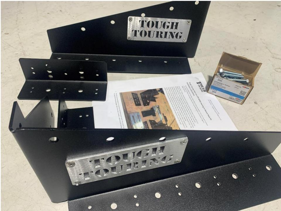
1. The kit is pictured above has an 80mm outbound folded section on both the front and rear brackets, to ensure that correct positioning is achieved, the base needs to be installed flush with the rear of the rack... The 200 series wind fairing will foul on all awnings if the brackets are not positioned inward 80 mm from the rear as per the fold on the base of the brackets.
