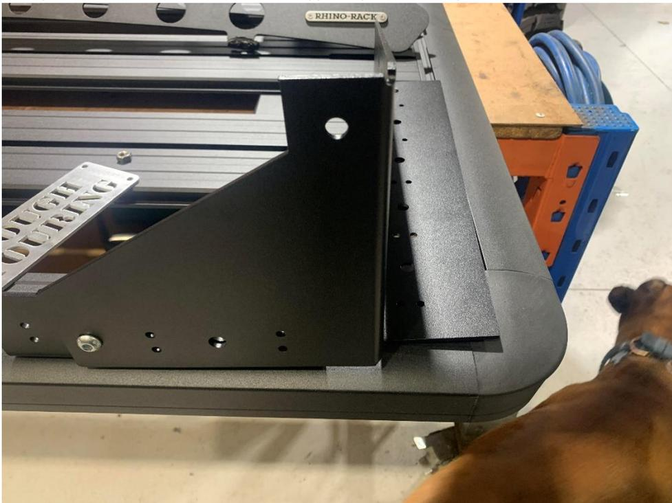
5. Take the rear passenger corner bracket (the one Pictured above) and loosely attach (Finger tight Bolt on the inner folded angle bracket ) Put it on the rack where its going to go and have a look... .. test fit this first. It is best fitted flush with the bottom edge.. In the Pic Above I've got it attached with one bolt forward about an inch of the face side of the bracket, as it lines up with two m8 bolts and 4 rivetts this way, as well as heaps of spots on the rhino rack.
