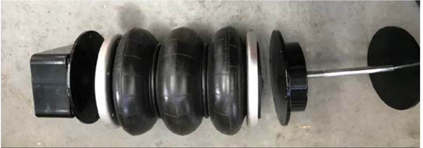
Exploded view of the air bag and Retaining plates – left hand side is the upper, right hand side is the lower.
